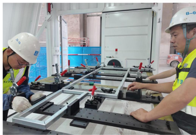
机械焊接工装 MECHANICAL WELDING TOOLING
